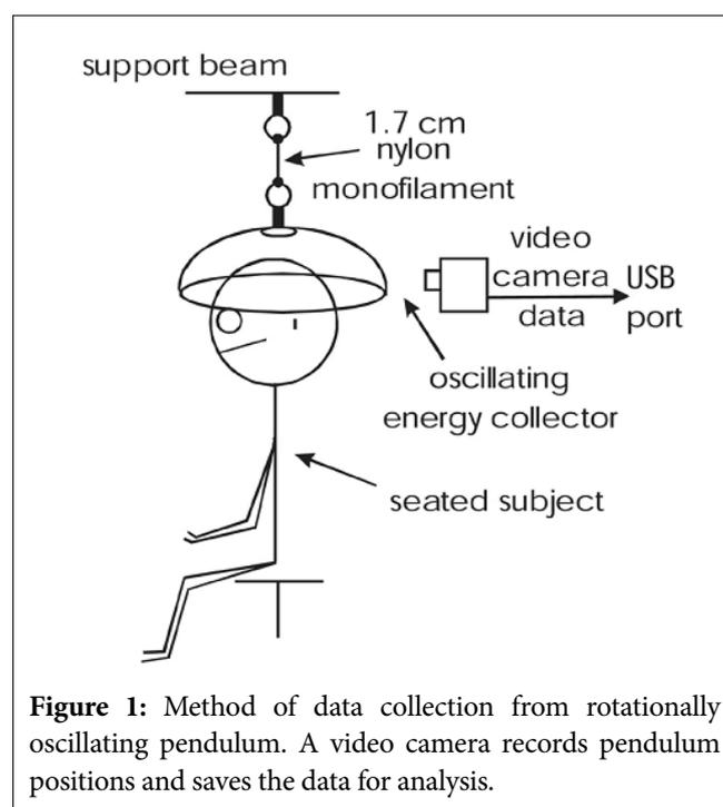
**Figure 1:** Method of data collection from rotationally oscillating pendulum. A video camera records pendulum positions and saves the data for analysis.
